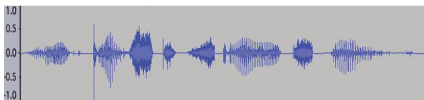
f0015 FIGURE 1.2 Temporal vibration pattern of the complex sound–pressure wave, when a male human voice utters the sentence: “Your Test Starts Now.”
